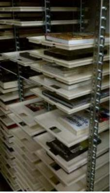
in metal columns in the storage bay. When items are returned or loaded, a tray is delivered to the induction window; the item and tray are then stored in the nearest available slot of sufficient height in the storage bays.
